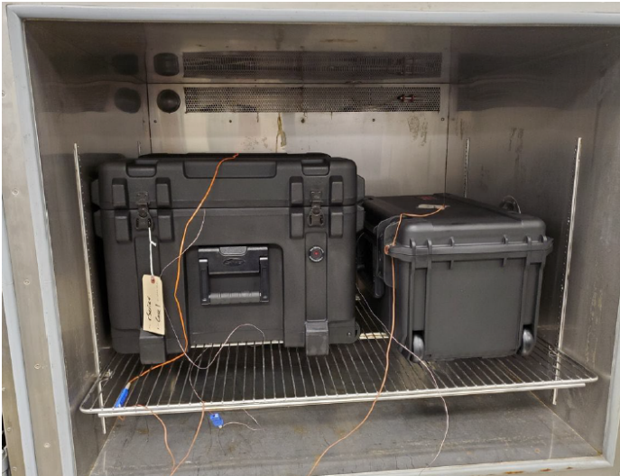
Figure 3: Temperature Shock Test Setup Chamber Example Note: iSeries Case is on the right
