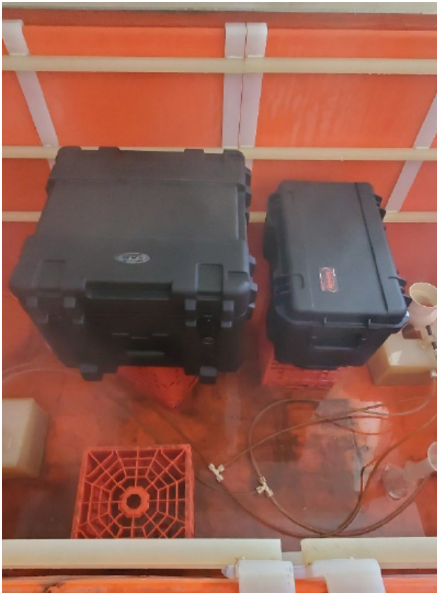
Figure 10: Salt Fog Test Setup Note: iSeries Case is on the right
