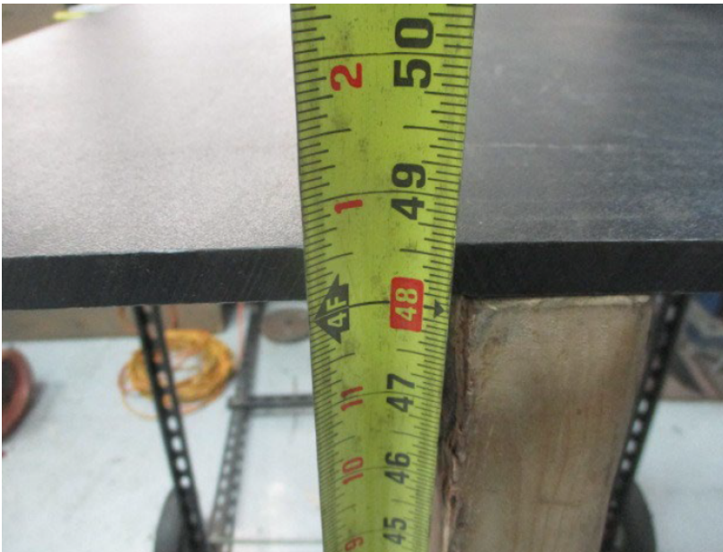
Figure 20: Transit Drop Height Verification
