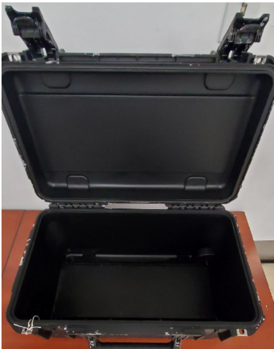
Figure 12: Salt Fog Post Test Interior – Prior to Cleaning
