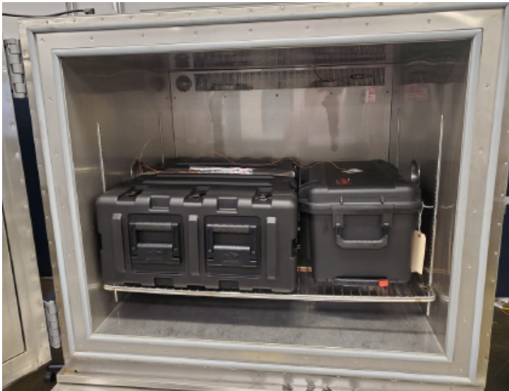
Figure 5: Humidity Test Setup Chamber Example Note: iSeries Case is on the right
