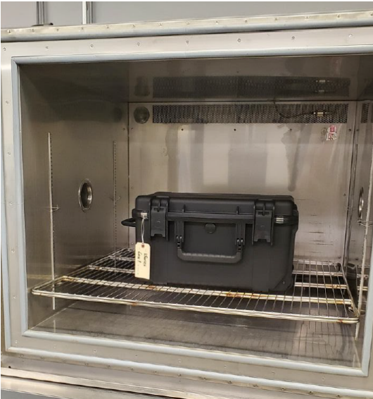
Figure 1: SKB iSeries Case in Low Temperature Test Chamber
